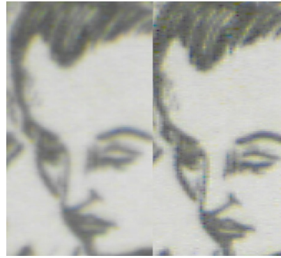
Figure 7. Comparison of sharpening filter applied to images and at zoom 500%. The left image has no sharpening filter applied and the right image has sharpening filter applied.
