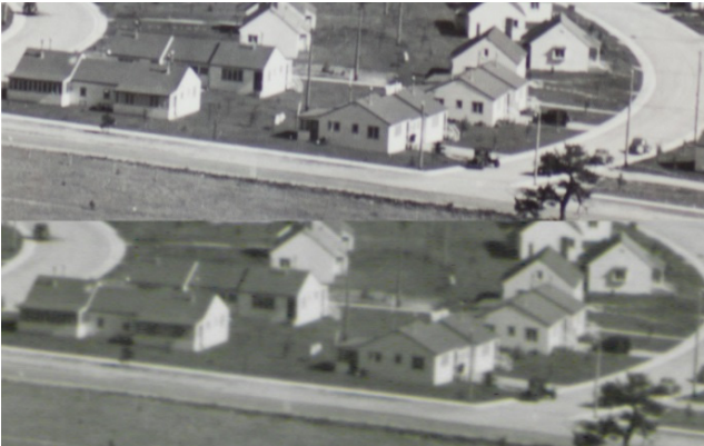
Figure 3. Screen view of at zoom 100% of a silver print. The top image was produced by the test DSLR camera and the bottom one was produced by our overhead scanner. Historical photograph from Colorado State University Archives and Special Collections.
